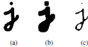
Figure 14: Binary image morphology: (a) original image; (b) dilation; (c) erosion
