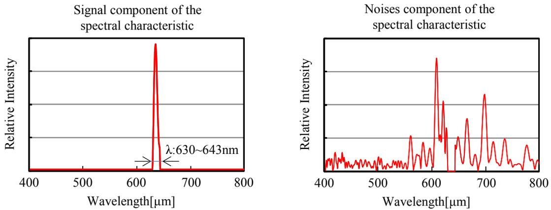
Figure 5. Extract signal component and the noises component from the obtained spectral characteristic
