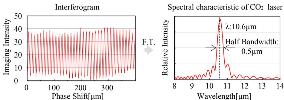
Figure 3. Obtained line spectrum of CO<sub>2</sub> laser by proposed portable mid-infrared Fourier spectroscopy apparatus
