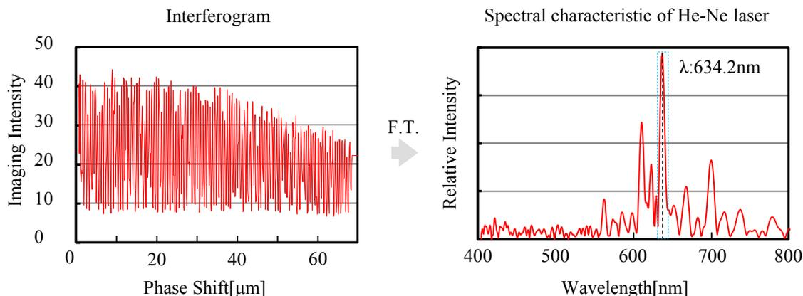
Figure 4. Obtained line spectrum of He-Ne laser by proposed portable Fourier spectroscopy apparatus
