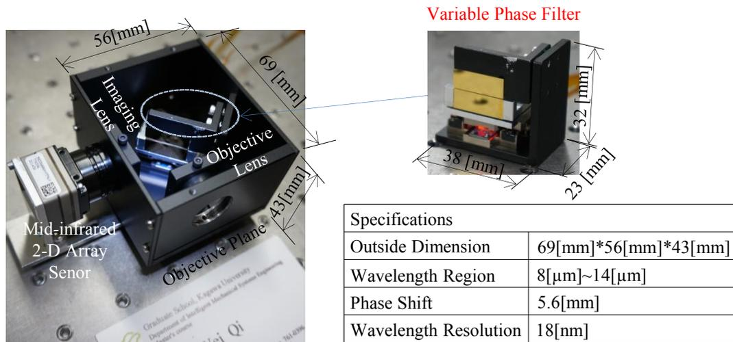
Figure 2. The portable mid-infrared Fourier spectrometer and specifications
