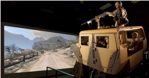
Figure 2. Armoured vehicle plugged in to training simulator
