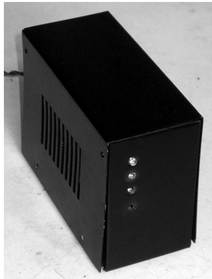
Figure 4.6 – Unit containing warning deciding circuit and main power supply.
