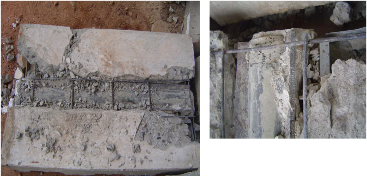
Figure 4.16: Configuration 2 Failure Surface
