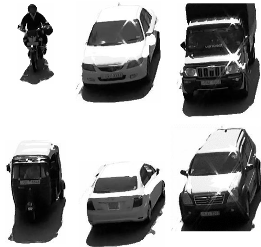
Figure 2: Irregular shaped vehicular segments obtained using recursive image segmentation algorithm
