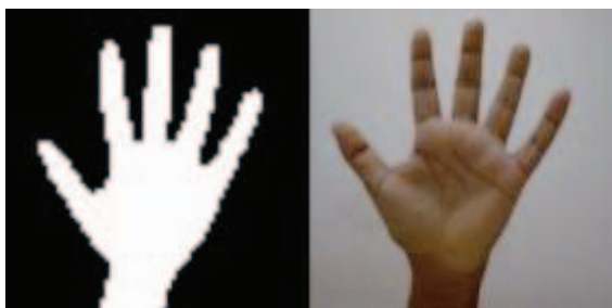
Figure 6: Hand Detection and Background Subtraction
