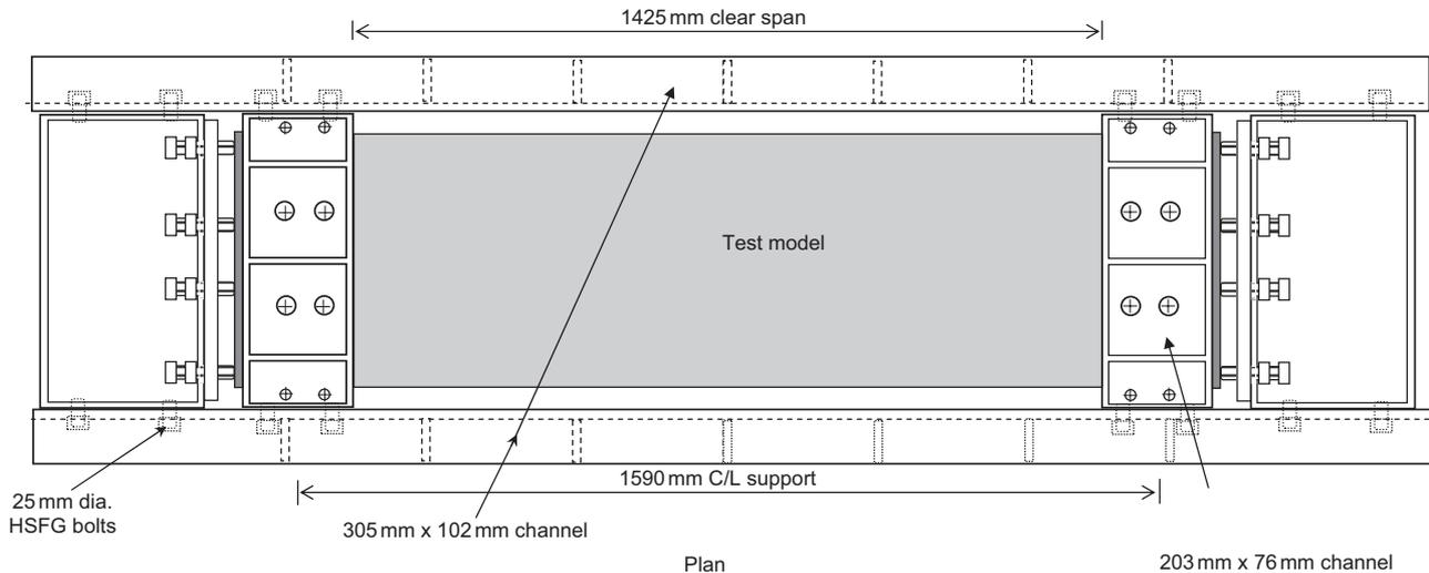
Figure 2. Plan view of the test arrangement to test in-plane restrained slabs; CL – centre line; HSFG – high-strength friction grip
