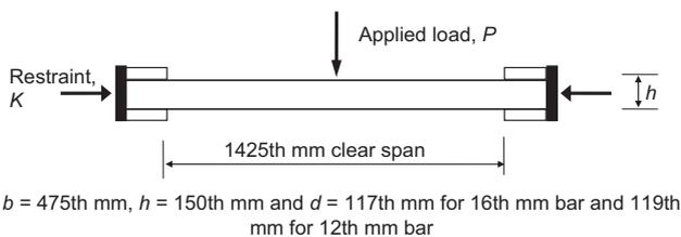
Figure 3. Test slab set-up
