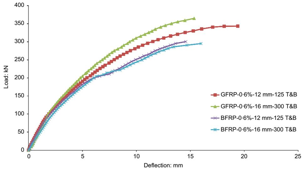
Figure 4. Load against deflection behaviour of the test slabs
