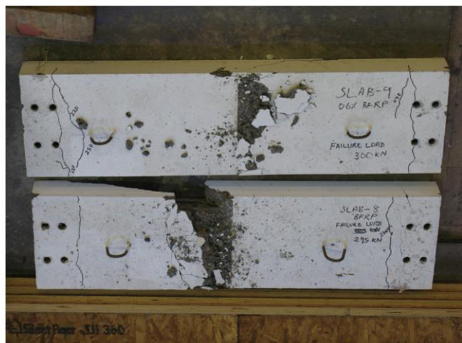
Figure 6. Crack on top surface and failure mode of FRP reinforced restrained slabs
