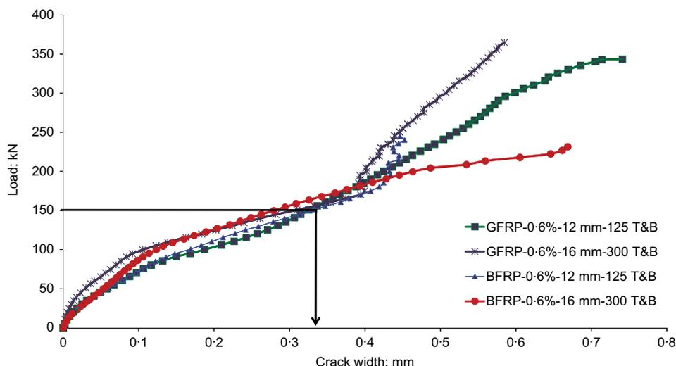
Figure 5. Crack width expansion with load increment
