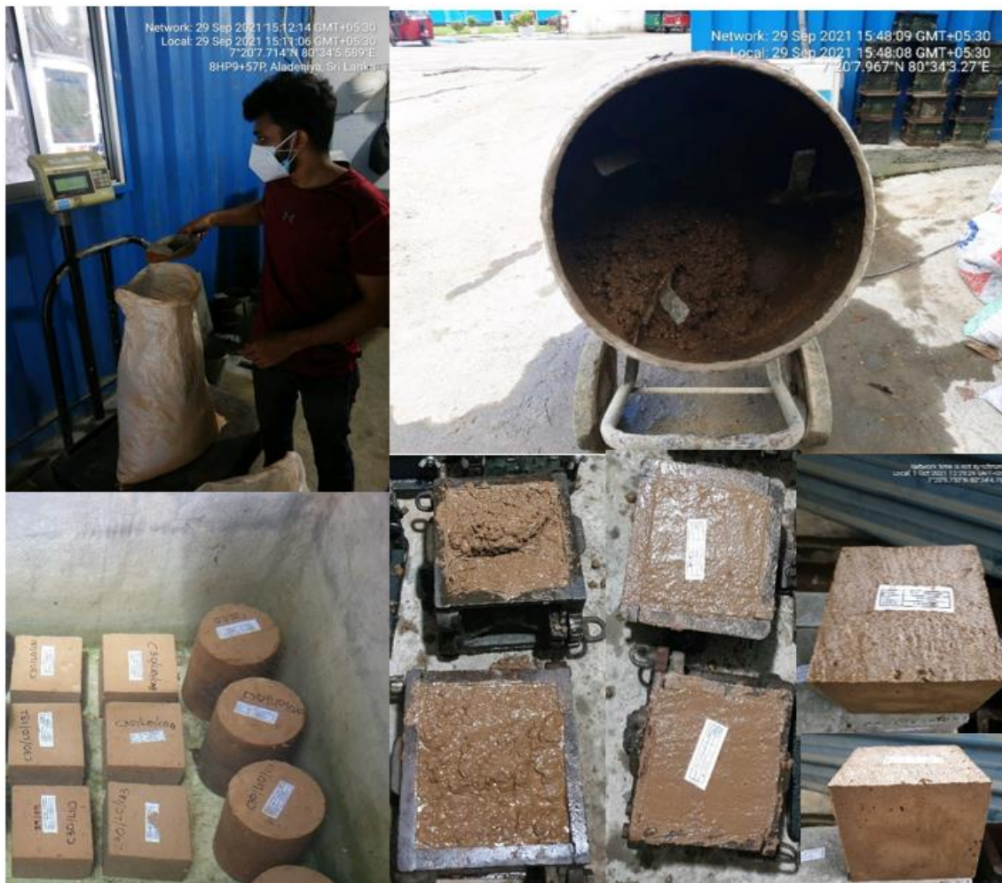
Figure 3.1 Concrete Casting and Curing
