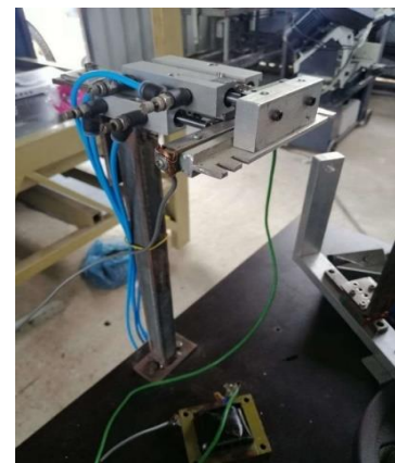
Figure 19. Mechanical structure of the sealing section
