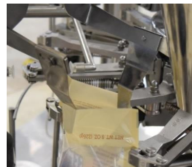
Figure 1. Packet Opening Jaws
