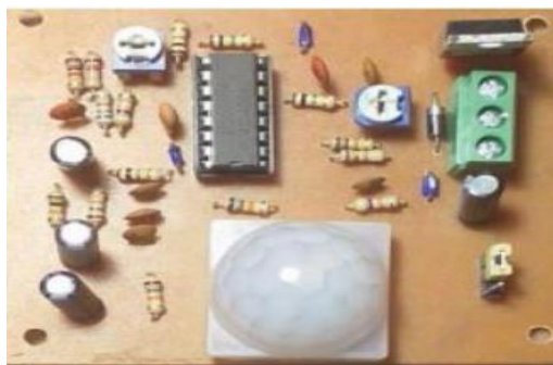
Figure 7. Constructed PIR sensor module
