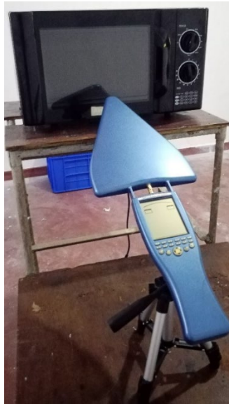
Figure 1. Spectran HF6065 spectrum analyzer with the microwave oven used for the study.
