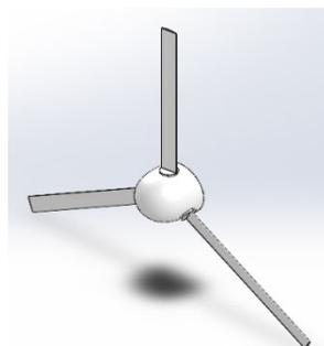
Figure 1: Depiction of novel rotor design used in simulating aerodynamic noise levels
