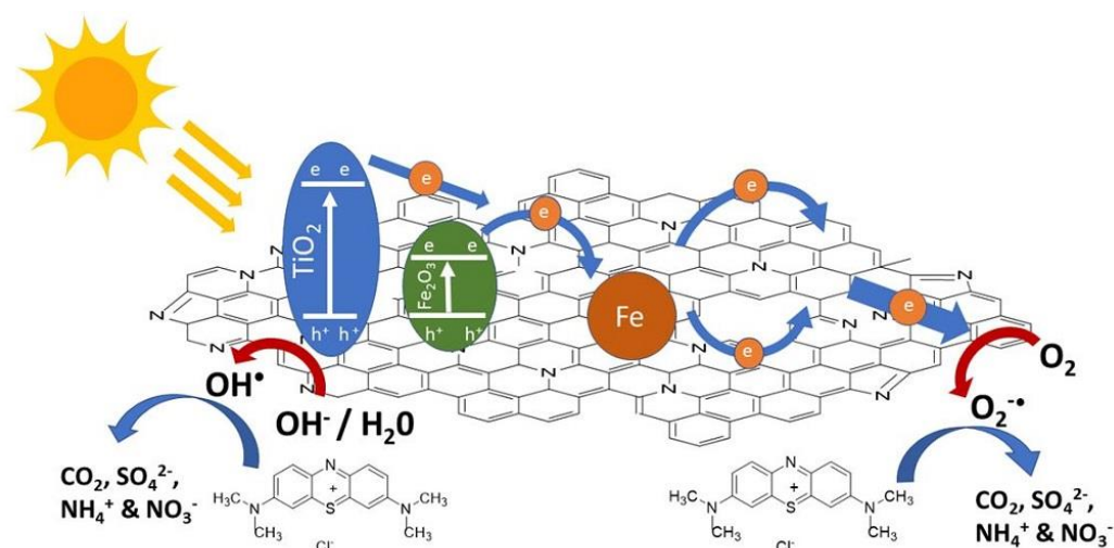
Figure 14. Mechanism of photocatalysis.
