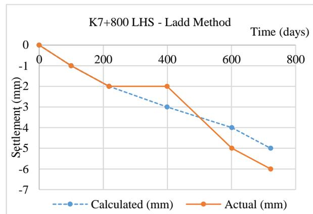
Figure 7: Settlement during DLP using the Ladd method for K7+800 LHS
