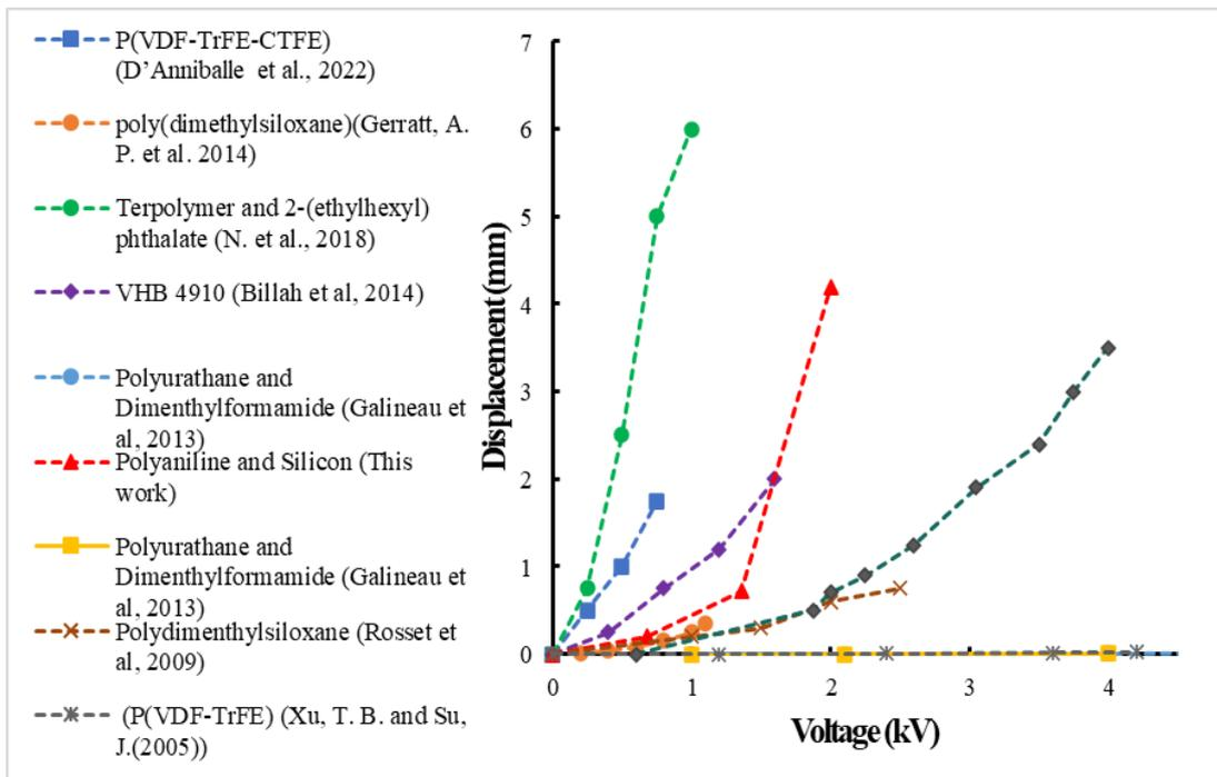
Figure 07: Comparison of deflections generated by different actuators
