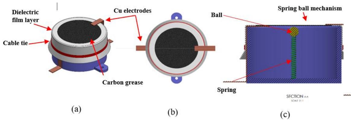
Figure 02: The schematic of the spring-loaded actuator (a) front view (b) top view (c) cross-sectional view
