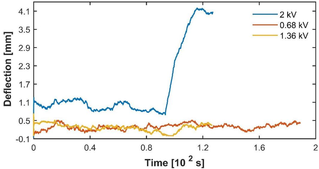
Figure 06: The variation of actuator deflection with time at different voltages
