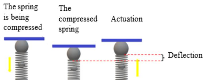
Figure 03: Schematic diagram of the working mechanism of the spring-loaded actuator
