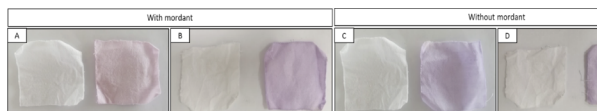
Figure 4: Scoured cotton fabric dyed with purple pigment extracted from BPU. 1 st dyeing: (A) & (B) with mordant, 2 nd dyeing: (C) & (D) without mordant
