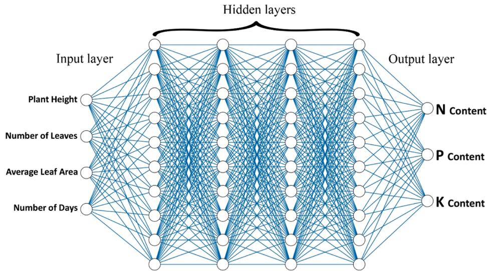
Fig. 1. Architecture of the DNN model.
