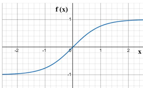
Fig. 4. Graph of the standard TanSig transfer function.
