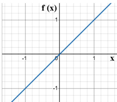
Fig. 3. Graph of the standard PureLin transfer function.
