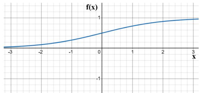
Fig. 2. Graph of the standard LogSig transfer function.
