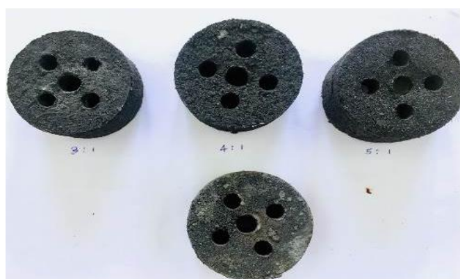
Figure 2 Honeycomb type pine-biochar briquette
