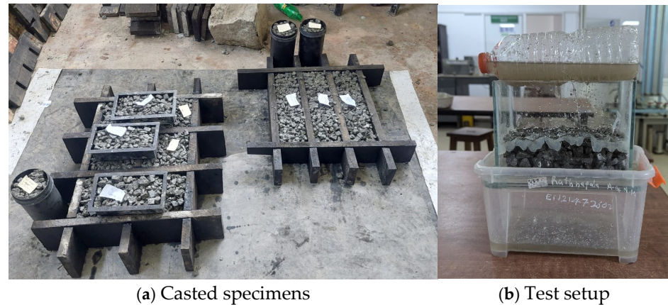
Figure 2. Test specimens and stormwater runoff filtration process.
