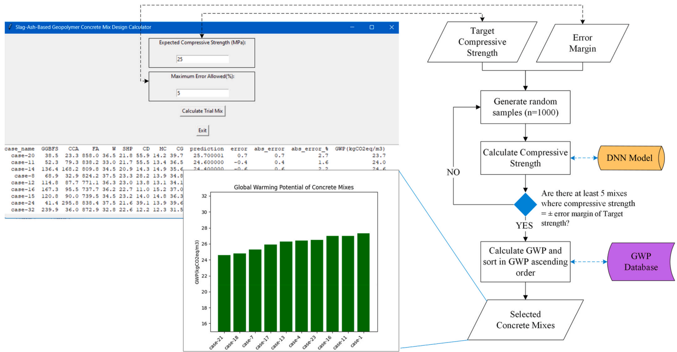
Fig. 12. The novel software tool to obtain a mixed design of slag ash-based geopolymer concrete with its global warming potential.
