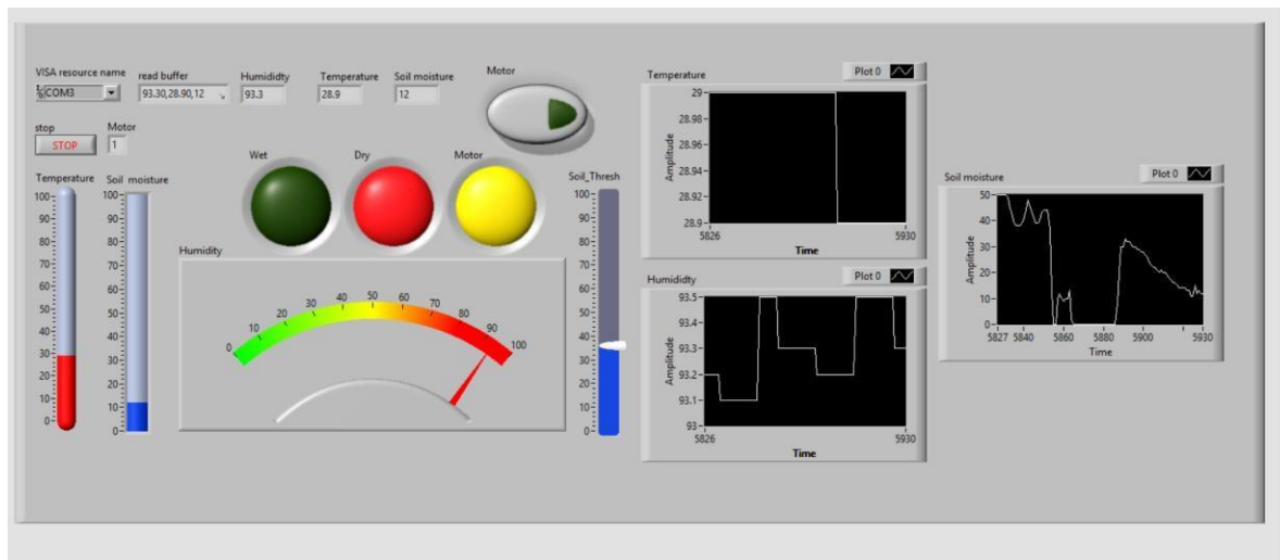
Figure 8: This figure shows a critical moment on the LabVIEW front panel where the automated system has activated the pump.
