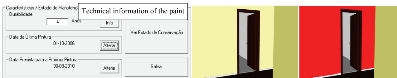
Fig. 10 Coating chromatic alteration according to deterioration state of the paint.
