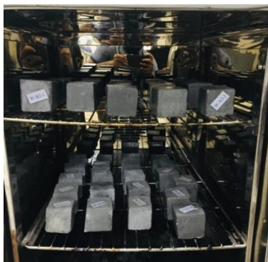
Figure 3. Drying of Samples
