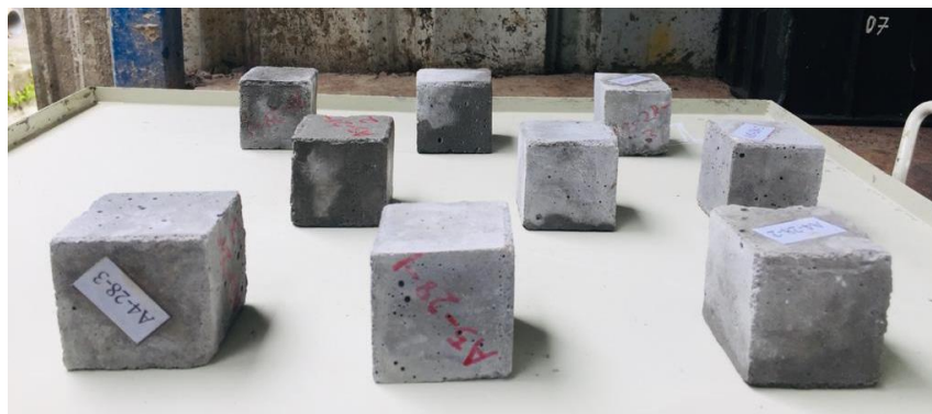
Figure 1. Hardened mortar samples
