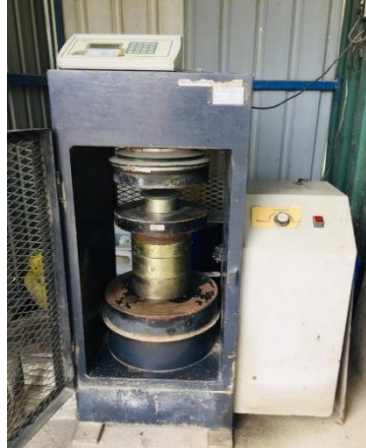
Figure 2. Standard compressive strength apparatus
