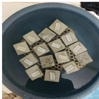
Figure 4. Immersion of Samples in Water
