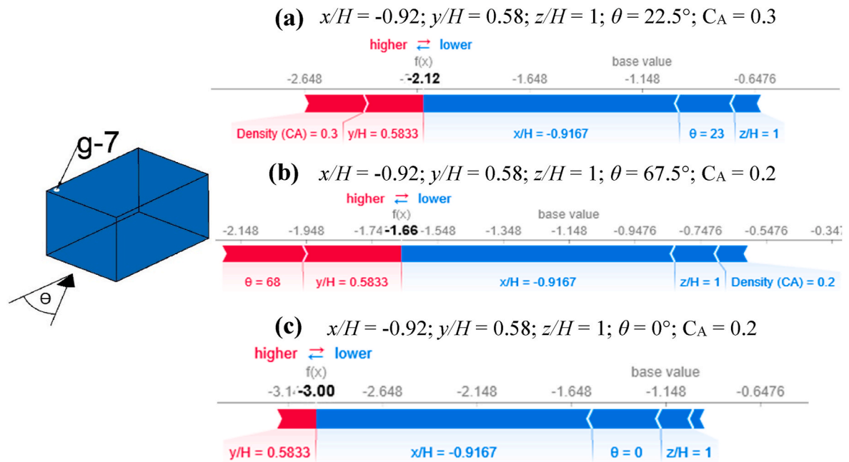
Fig. 15. SHAP local explanation for C_{p,min} of the pressure tap (g7) for (a) \theta = 22.5^\circ and C_A = 0.3 , (b) \theta = 67.5^\circ and C_A = 0.2 , and (c) \theta = 0^\circ and C_A = 0.2 ( \theta – wind incidence angle; C_A – area density).
