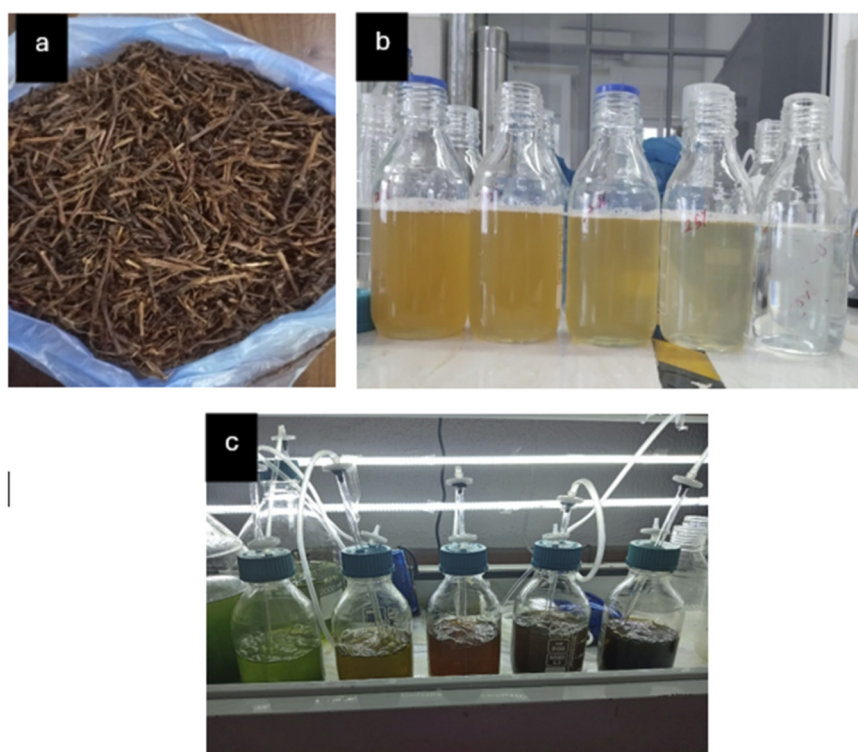
FIGURE 1 Representative images of (a) raw tea stem waste, (b) hydrolysate at different dilution levels, and (c) microalgal cultivation setup 2.4.2. Phase II: Main Cultivation.
