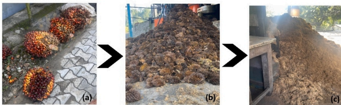
Fig. 1. Pre-treatment process of empty fruit bunches. a) harvested fruit bunches, (b) de-fibred bunches, and (c) processed fibres.
