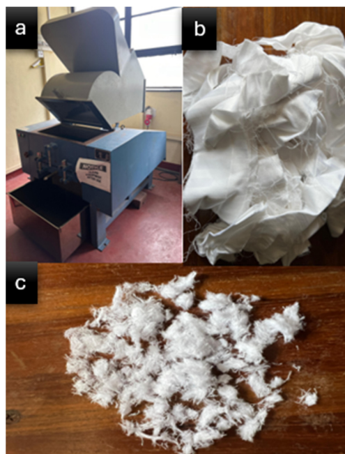
Figure 2. Mechanical processing sequence of post-industrial textile waste: (a) The rotary shredding machine utilized for fiber size reduction; (b) Raw textile waste off-cuts prior to processing; (c) The resulting shredded fiber mass after the second shredding cycle, illustrating the degree of fiber disentanglement and fluffing used for composite fabrication.
