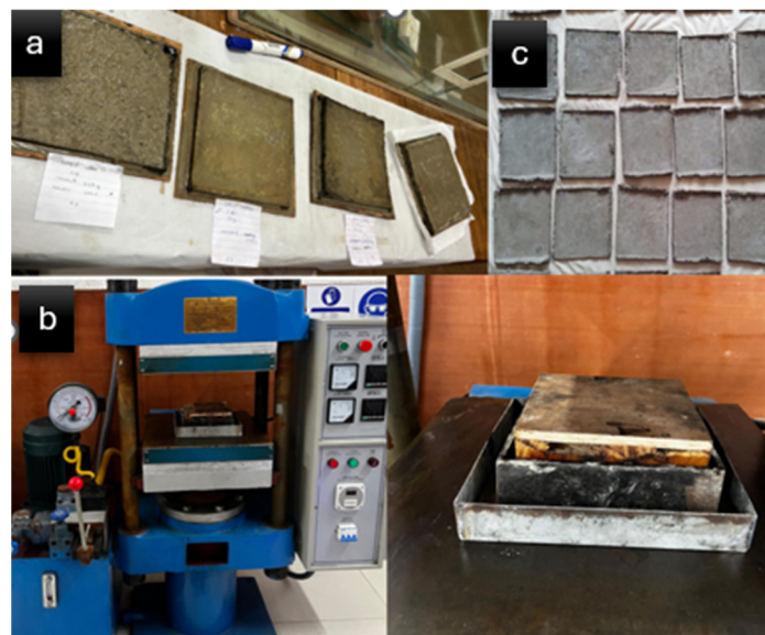
Figure 3. Fabrication process of the ceiling sheets: (a) Fresh fiber–cement mixture placed in 150 \times 150 mm steel molds; (b) Hydraulic compaction of the specimens at 2 MPa; (c) Demolded specimens during the initial curing phase.
