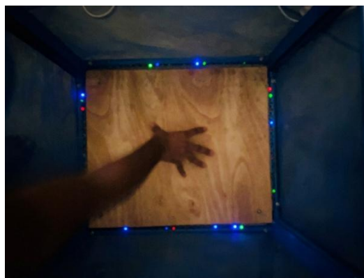
Figure 26 – LED illumination under (simulated) applied footstep load
