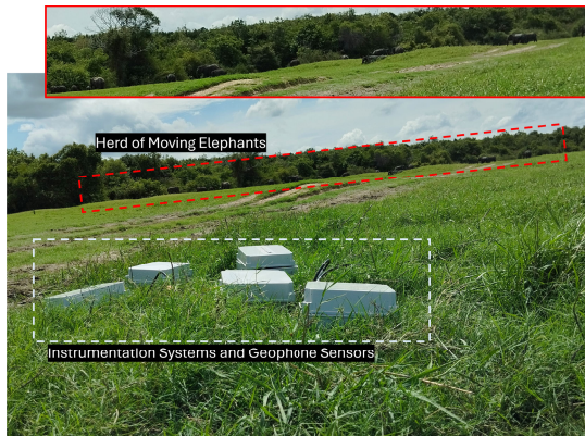
FIGURE 6. Sensor and instrumentation system placement in the field study at Kawudulla.
